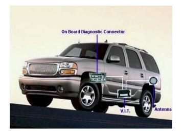
Installation is quick and simple. The Ward Fleet Data System has two leads, a plug-in lead to the OBD connector and another to the filler neck antenna that attaches to the tank filler neck. This eliminates splicing into wiring harnesses or other closed systems to obtain power and odometer values. Installation time is greatly reduced and intrusive warranty issues are eliminated.
