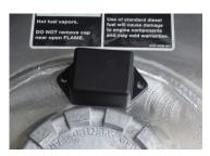
The Fuel Tag works in conjunction with the Ward Hose Module for automated fueling access. Easily programmed, its unique ID ensures only specified assets can initiate fueling and receive the correct fuel type and volume.
