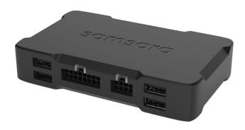
The **VG54-NA** Vehicle Gateway is an advanced sensor platform for fleets, providing operators with real-time location and analytics, sensor data, accessory compatibility, Wi-Fi hotspot connectivity, and ELD-ready hours of service logging.
